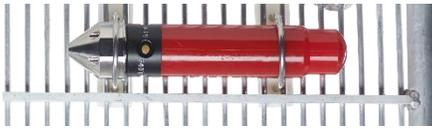
Echo (aside) was developed for the shrimp fishery as there was no reliable way to detect shrimp. Notus cooperated with fishermen on the west coast of the USA to develop the system. Basically, when shrimp hit the grate, they make a very distinctive sound. Echo listens for this sound and transmits the data back to the vessel wirelessly to be displayed on a graph. **Echo doubled and sometimes tripled catch rates.**
